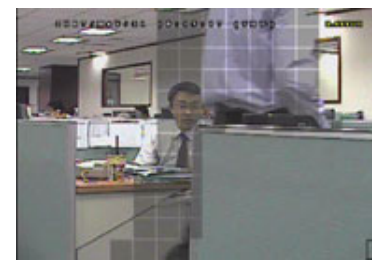
When any movement is detected, you will see the grids are flashing.
